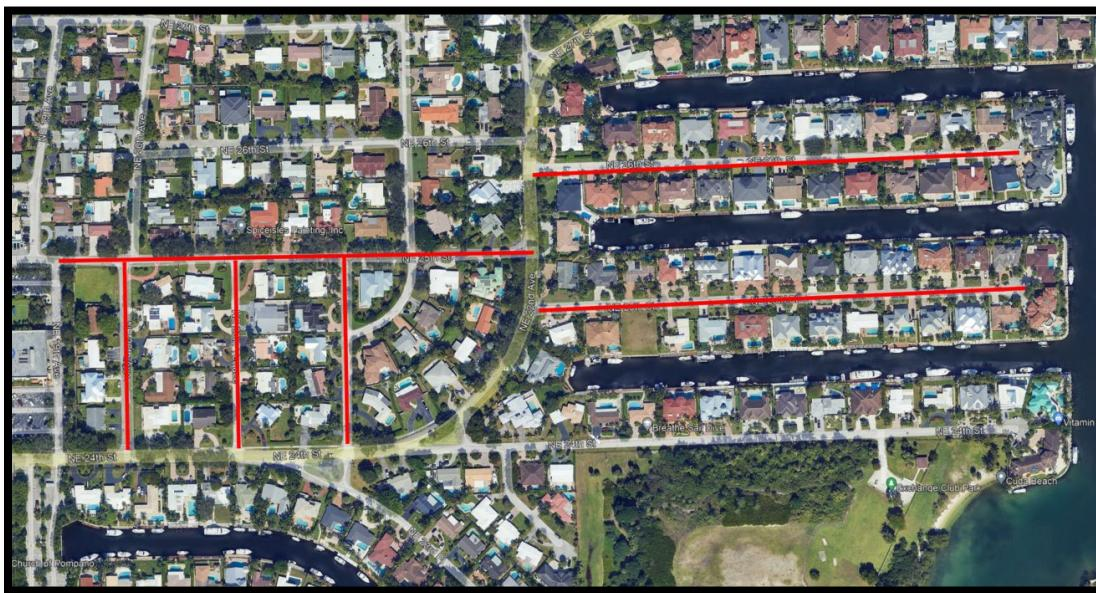
To minimize inconvenience to Pompano Beach customers, MPC will employ a trenchless technology method known as Horizontal Directional Drilling (HDD). This method allows the pipe to be replaced without excavating the entire route of the pipeline. However, minor excavations will occur at the placement of each meter upon the property. Any disturbed areas will be restored to original condition.
